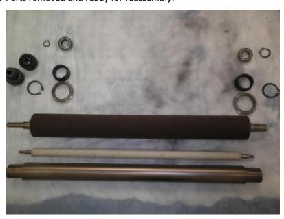
16. Place foam pressure roller and heat roller inside new belt:
