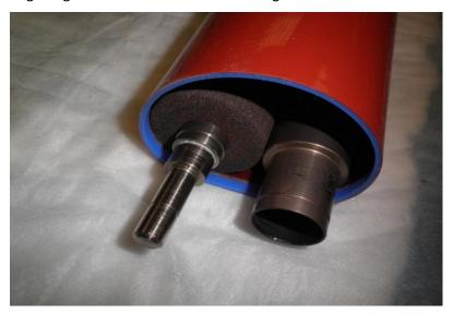
18. Grasping the ends of the heat roller, drop the foam pressure roller into its frame opening:
