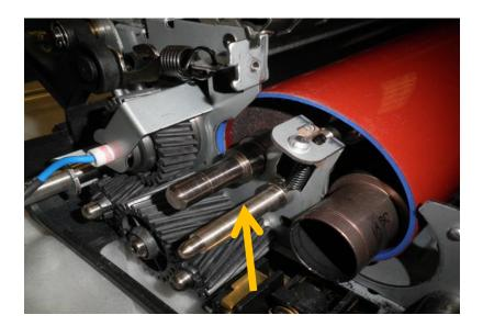
23. Install bearings on both ends of the foam pressure roller:
