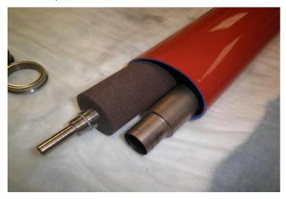
17. Align large diameters of rollers inside of guide ribs:
