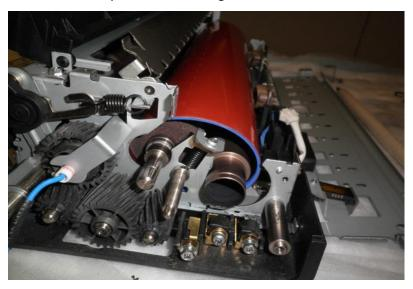
20. Slide the tensioner roller into the belt so that it is resting on top of the heat roller:
