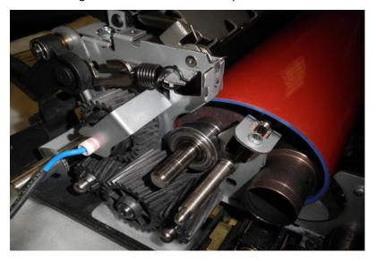
24. Install one-way clutch gear on foam pressure roller shaft. Metal edge of bearing should go toward the roller. When installed in the correct direction, it should drive the belt when turned in the clockwise direction viewed from the drive side:
