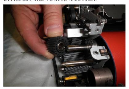
25. Install the bearings in the frame over the ends of the heat roller. Visually confirm that the belt is tracking properly on both ends of the heat roller (guide ribs not riding on large diameter):
