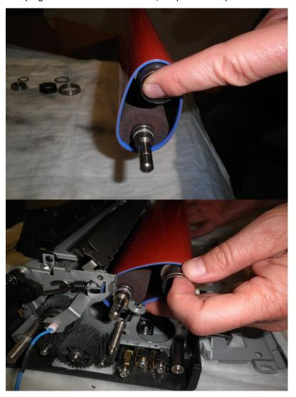
19. While applying tension to the belt, push the heat roller into its frame opening. Make sure both rollers are still in position between guide ribs:
